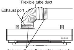
Taping with nonflammable materials (Aluminum tape, etc.)
