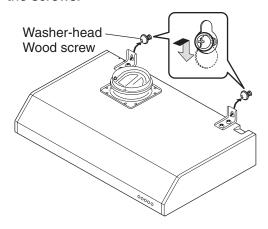
2) Put 2 washer-head wood screws to the rear of the cooker hood and tighten them securely.
